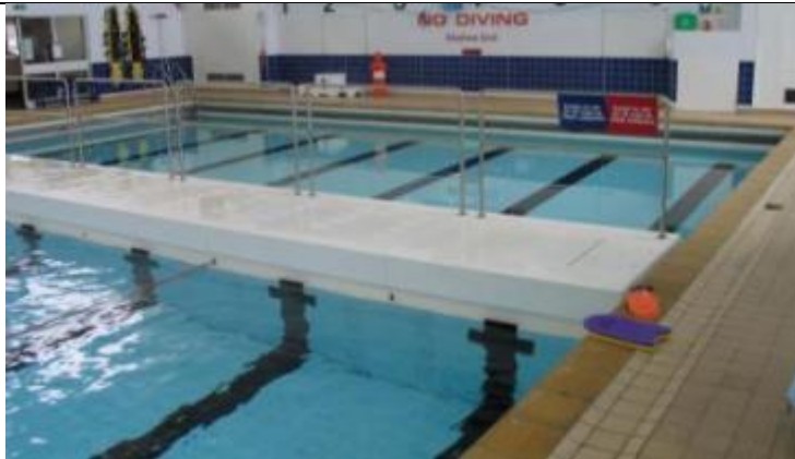
Fixed bulkhead (to create 25m pool plus learner pool)
