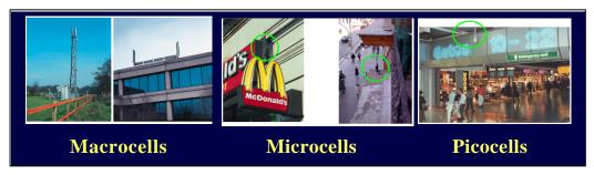
A macrocell provides the main coverage in a mobile network, having a typical power output of tens of watts. The antennas for these are normally mounted on ground-based masts, rooftops and other existing structures, positioned at a height that is not obstructed by surrounding buildings and terrain.
